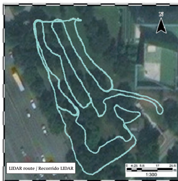
Figure 2. Portable LIDAR route in an urban forest at the Instituto Tecnológico y de Estudios Superiores de Monterrey (Nuevo León, Mexico) to obtain aerial biomass parameters.
